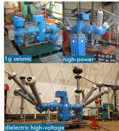
Figure 9: Clean Air Vacuum Blue GIS 145 kV / 40 kA / 3150 A / -50°C / 1g – Technical features
